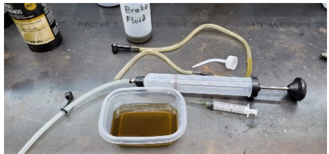
Photo 2 – Special tools recommended to perform fluid replacement. Small and large syringe, tubing and bottle to catch old brake fluid.
