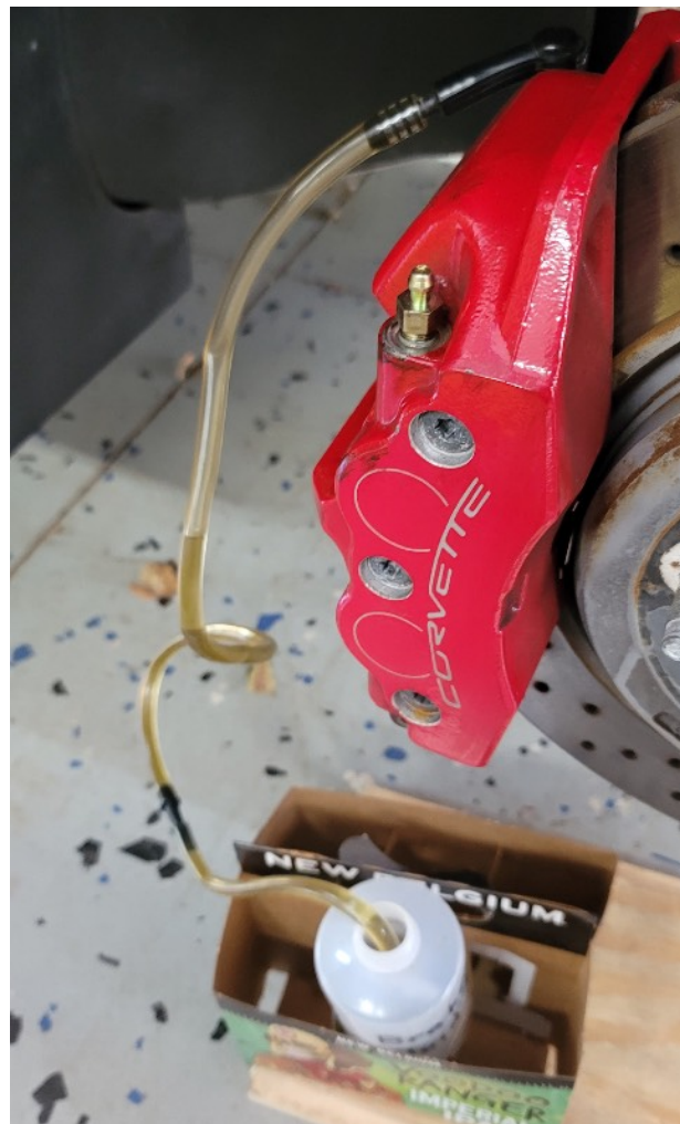
Photo 6 – Speed bleeder screw with nipple adapter with tube run to catch bottle.
