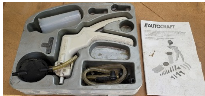
Photo 4 – Typical inexpensive auto parts store vacuum brake bleed system. Cost is less than $50.
