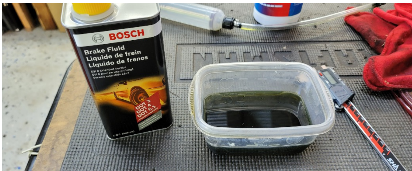
Photo 3 – Dirty brake fluid from the clutch and brake reservoir. Both were nearly black.
