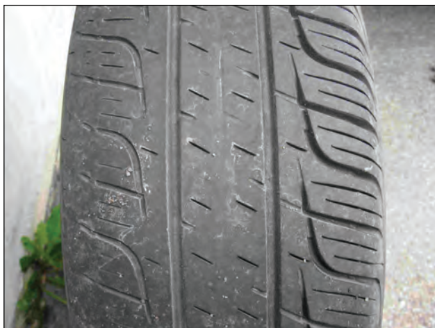
Tire worn on inside due to excess negative camber
