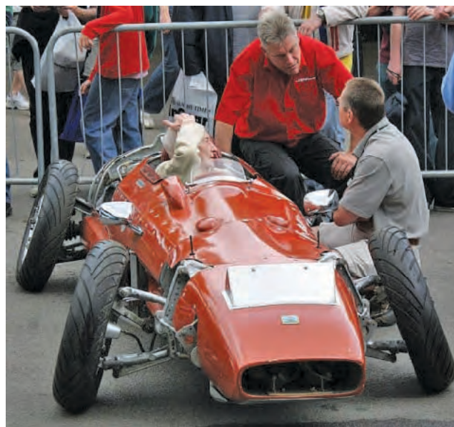
1960 Milliken MX1 with large negative camber
